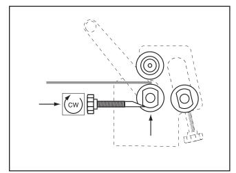
Figure 15. Raising bottom roller for flat rolling.
